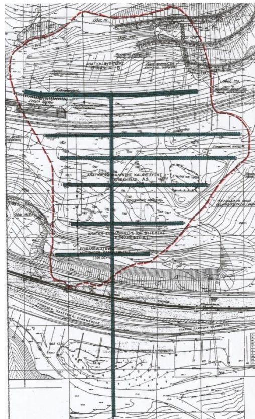
Plan view of drainage tunnels
