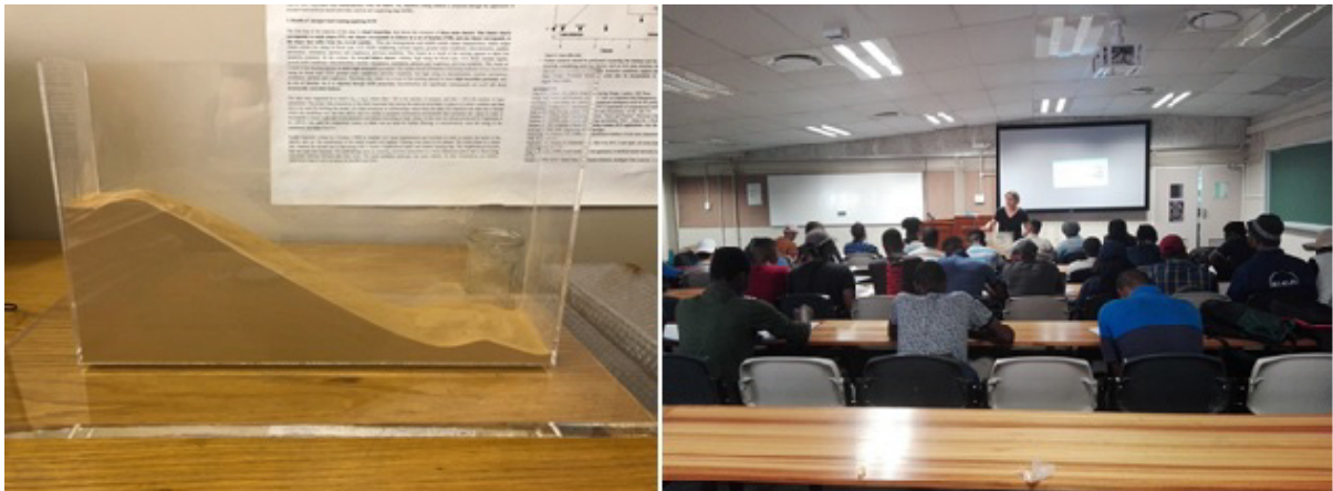
Figure 2. a) Slope model that served as a classroom model in order to show the repose angle of the dry sand slope, b) demonstration of function of reinforcement through the use of the small-scale model slope
