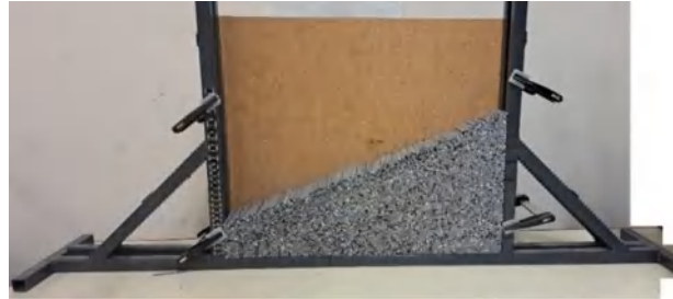
Figure 4. Natural slope of a rod assembly.
