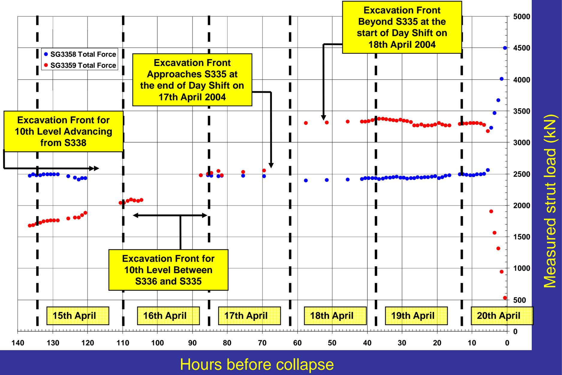
Change in Measured Load at Strut 335
