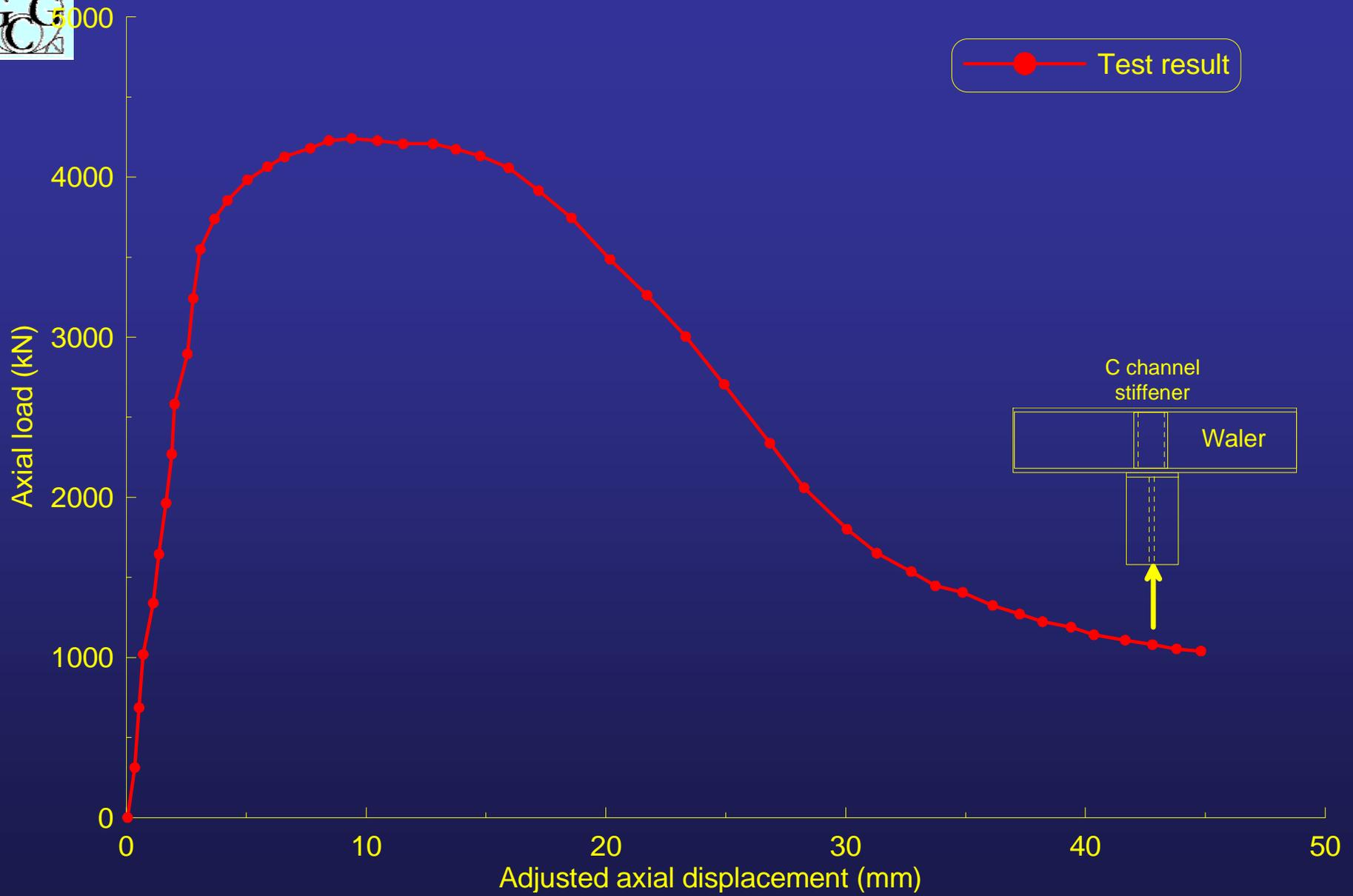
*Calibration of FE model of strut-waler connection*
