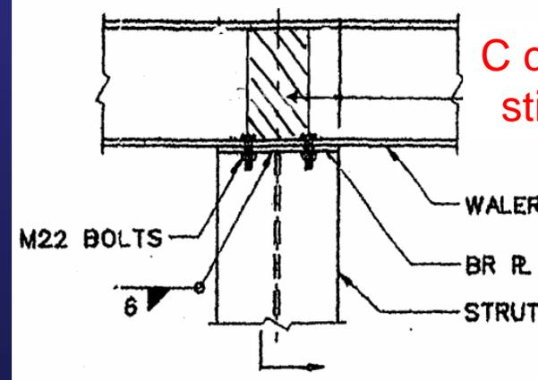
*Replacement of plate stiffeners at strut-waler connection*
