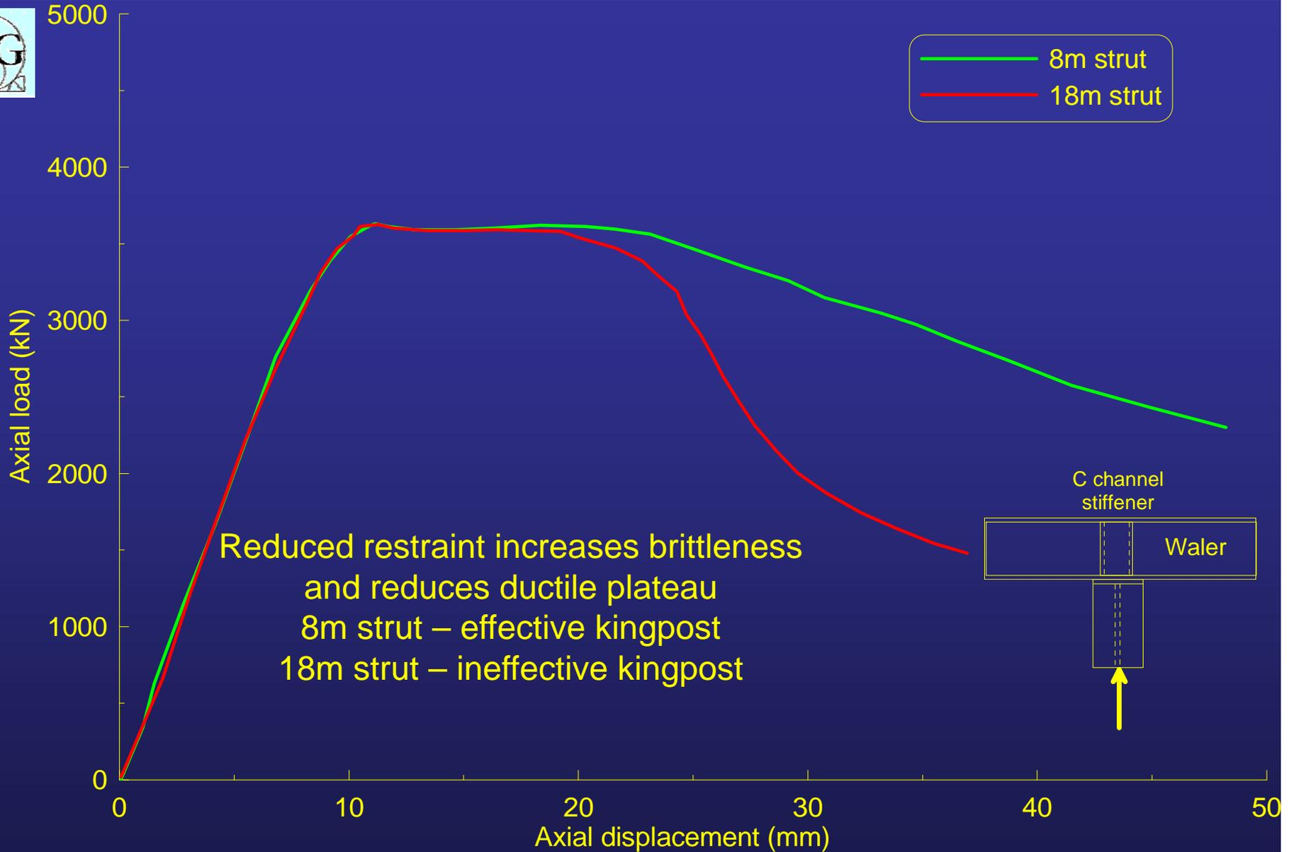
*Effect of strut length (bending restraint) on brittleness of connection*
