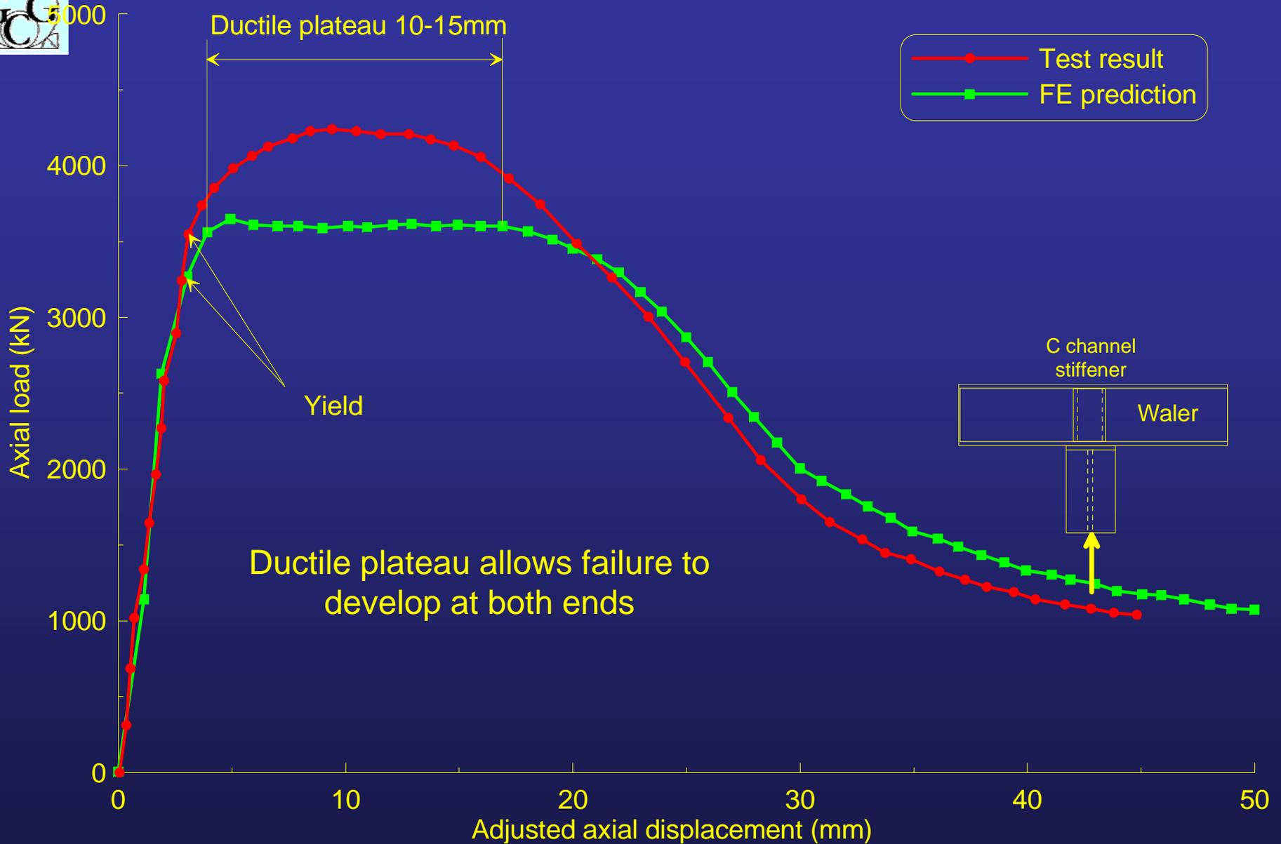
*Calibration of FE model of strut-waler connection*
