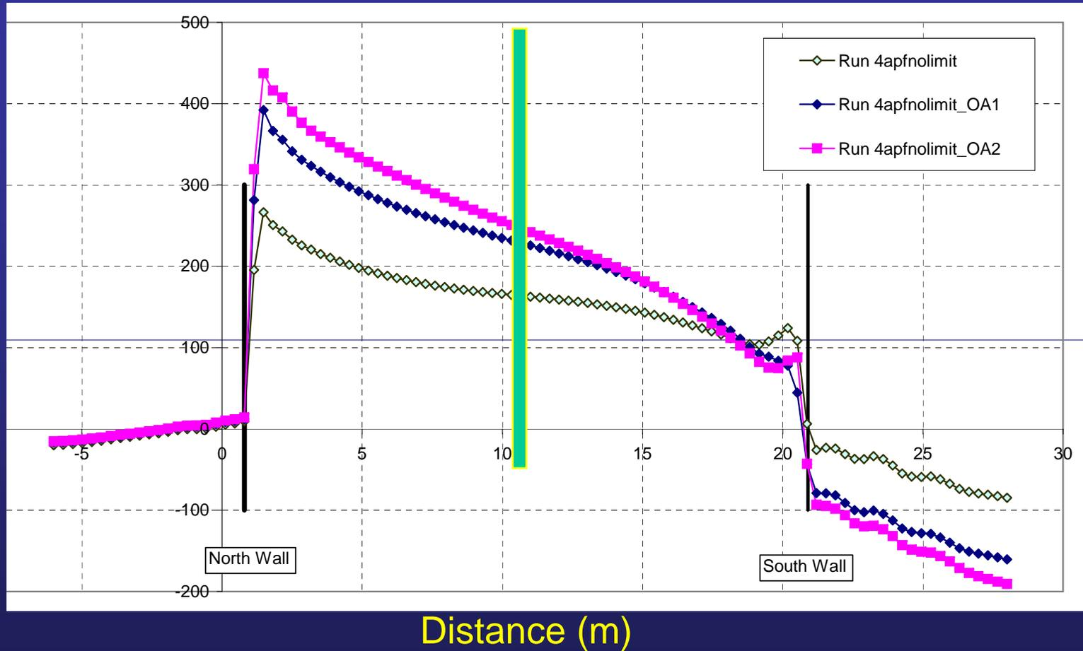
*Predicted vertical displacement of lower JGP layer after excavation to 10<sup>th</sup> level*
