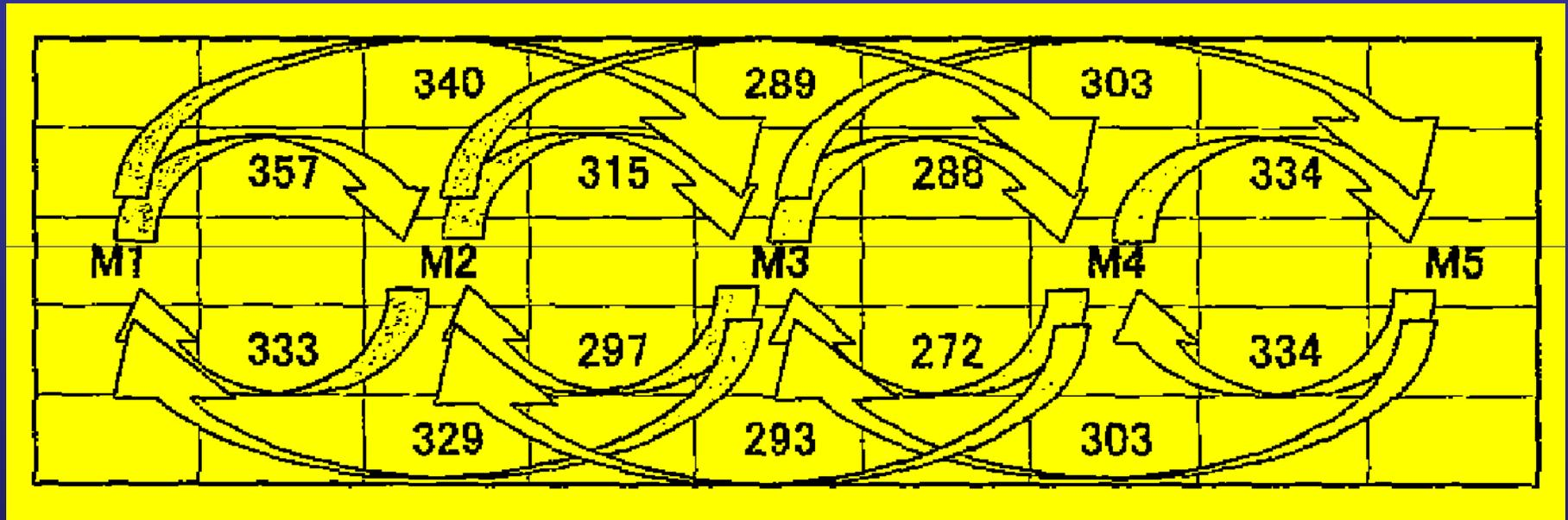
*Shear wave velocity measurements in JGP at Type K*
