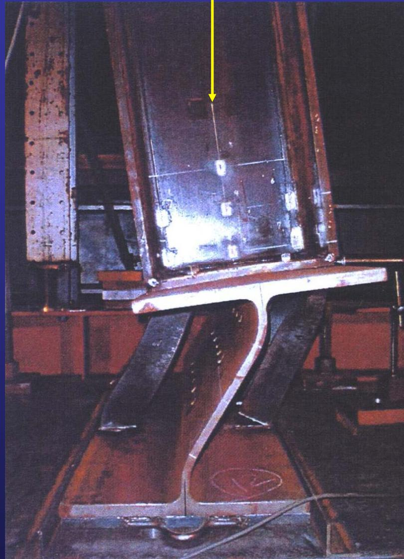
*Test on C channel stiffened connection by Nishimatsu*
