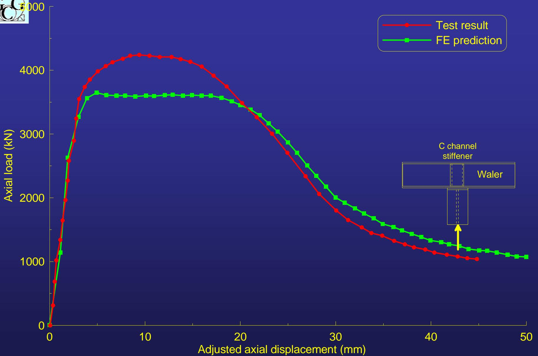
*Calibration of FE model of strut-waler connection*
