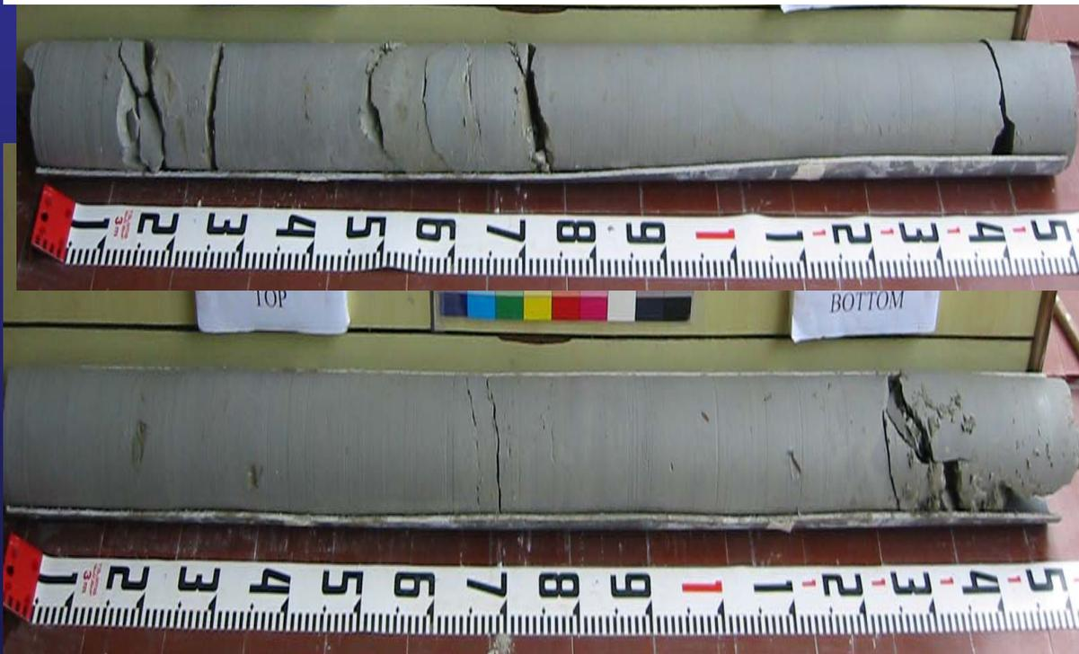
*JGP quality in 100mm cores from borehole M1 in Type K*
