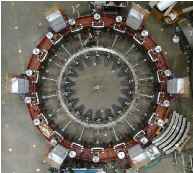
Figure 1. View from above of the test set-up for loading the halfscale model segmental ring (larger outer ring is the reaction ring)
