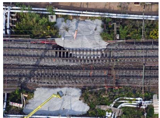
Concrete backfill into the collapsed Rastatt TBM rail tunnel
