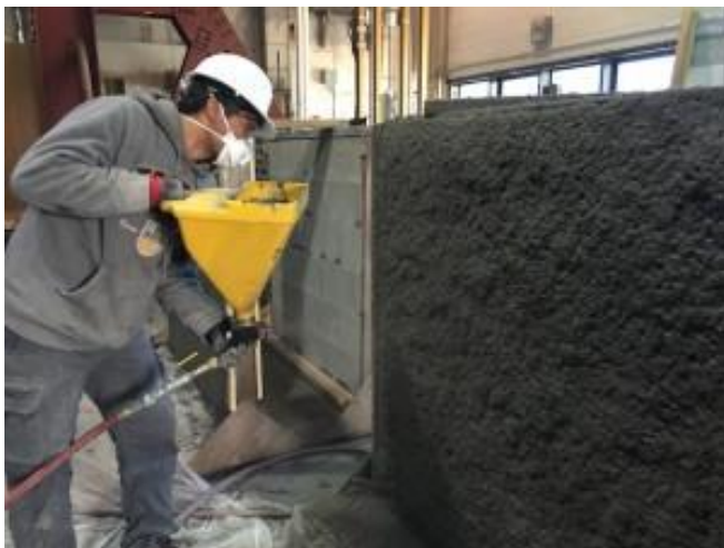
The EDCC getting sprayed on a block wall in the UBC lab.
