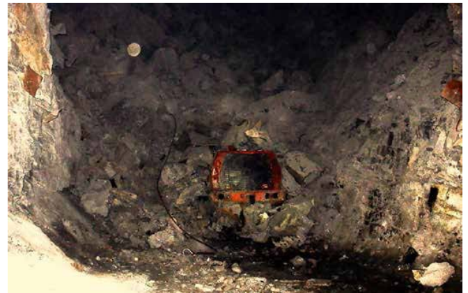
Fig. 4 - Mechanised equipment damage by rock falls in open stopes (after Le Roux, 2015)
