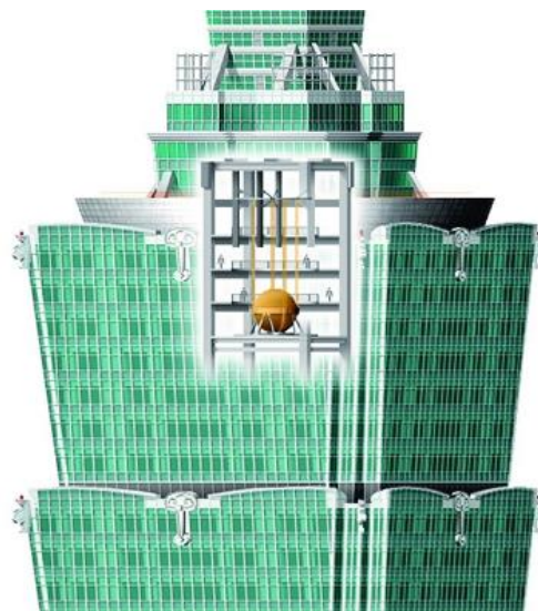
The main tuned mass damper in Taipei 101 sits above the 87th floor
