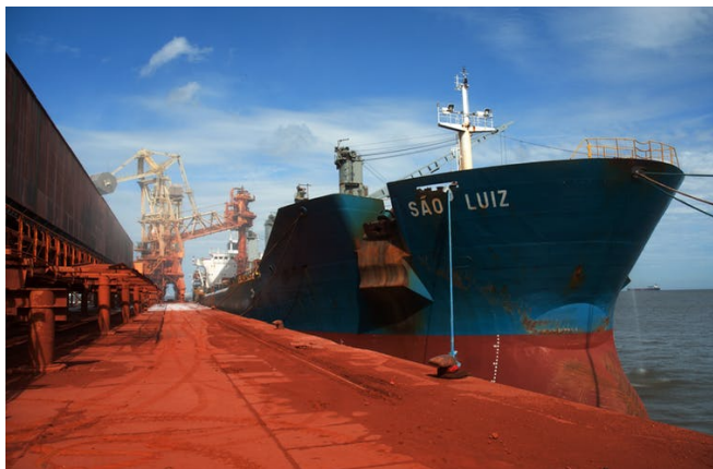
A cargo ship being loaded with bauxite.
