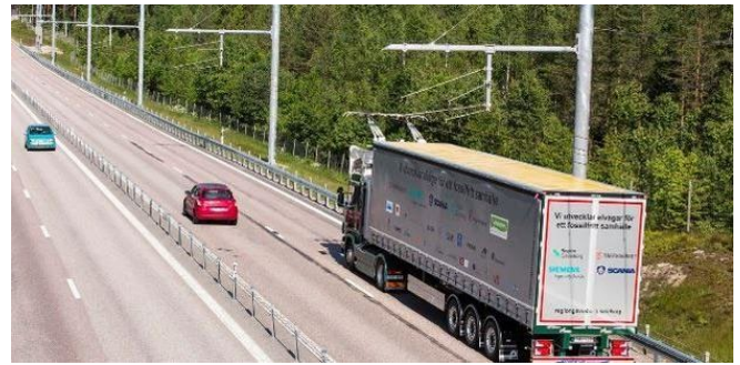
Sweden's Highway E16 has become the first in the world to include a 2.0 mile-long eHighway. Scania Group
