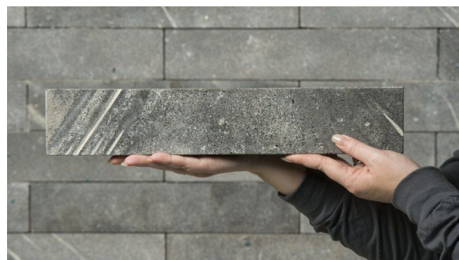
Bio-cement start-up BioMason grows bricks out of sand and bacteria
