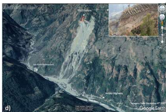
Historical satellite imagery of the Jure landslide: a) Multiple rockfall/rock slope failures occur throughout the slope and highway, 2004; b) Rockfalls and large mid-slope landslide
