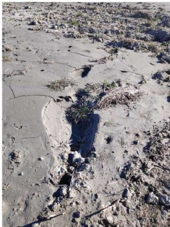
FIGURE 14. DETAIL OF EJECTED SAND ALONG A CRACK.
