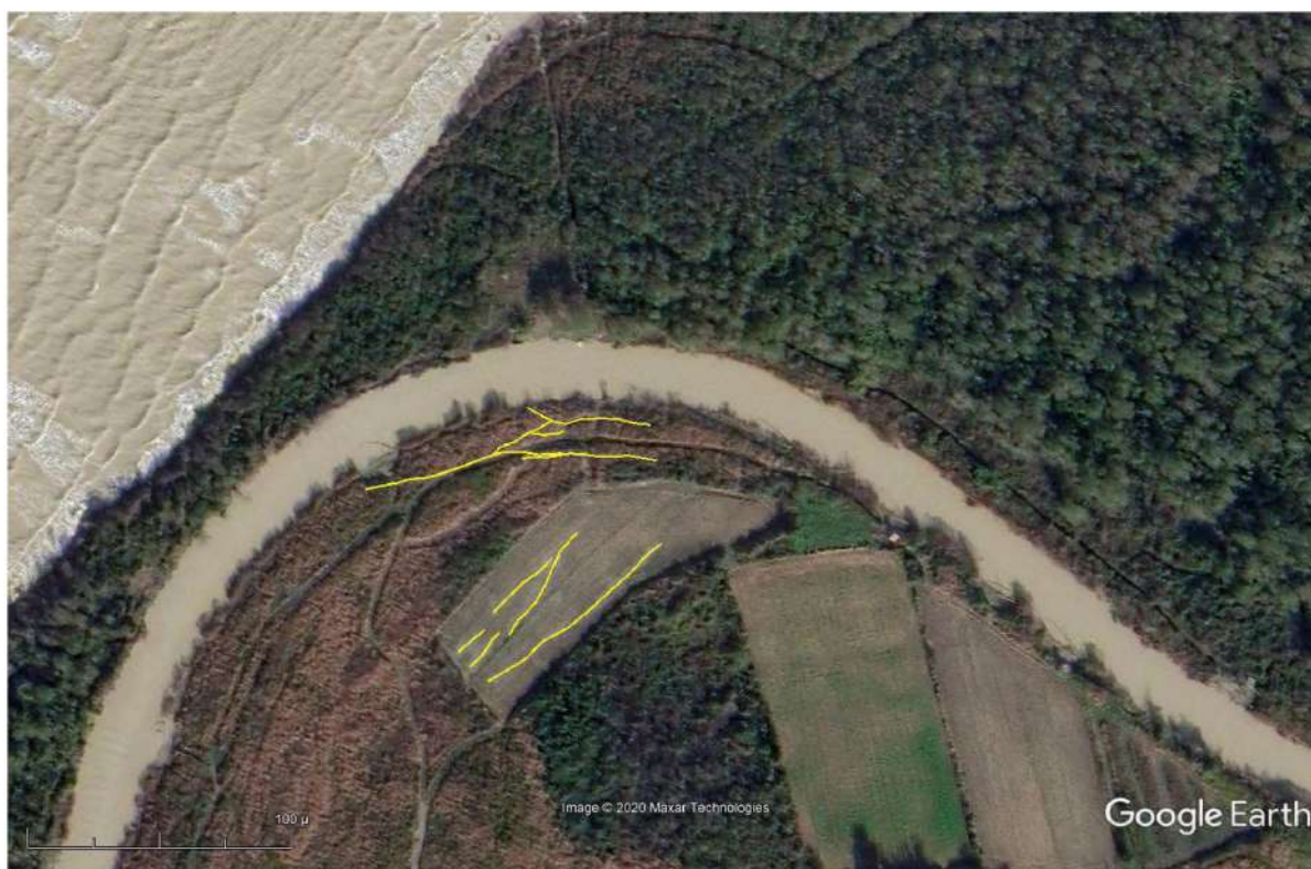
FIGURE 12. MAPPED LATERAL SPREADING NEAR THE RIVER ESTUARY IN AREA 2. LIQUEFACTION WAS WIDESPREAD ALONG THE SOUTHERN BRANCHES.
