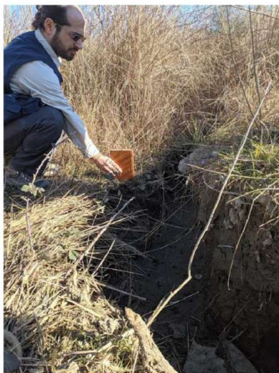
FIGURE 16. VERTICAL DISPLACEMENT OF UP TO 15 CM WAS EVIDENT IN CERTAIN PLACES ALONG THE CRACK.
