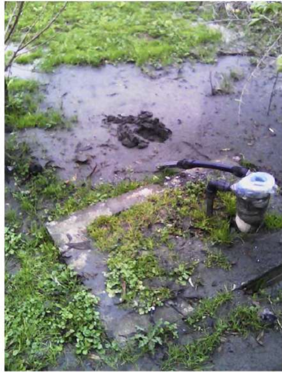
FIGURE 18. ACCORDING TO REPORTS, LIQUEFACTION AT THIS SITE STARTED WITH GRAVELS THAT WERE EJECTED FIRST, FOLLOWED BY SAND. THE SAMPLING SITE IS ALSO VISIBLE.
