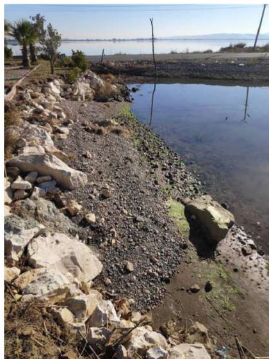
FIGURE 20. SMALL-SCALE MASS MOVEMENT DUE TO LATERAL SPREADING NEXT TO PATOK LAGOON.
