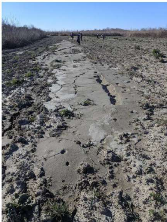
FIGURE 13. PART OF THE SOUTHERN BRANCHES OF THE LATERAL SPREADING NEAR THE RIVER ESTUARY.
