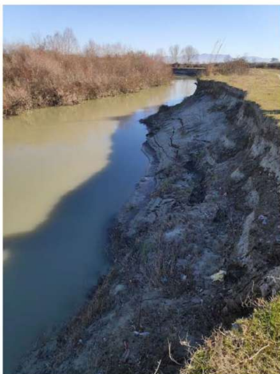
FIGURE 9. TYPICAL LATERAL SPREADING ALONG THE RIVERBANKS IN RRUSHKULL AREA.
