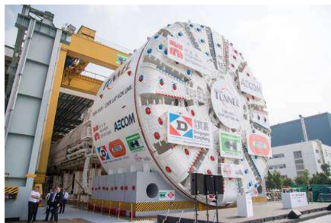
TM-CLKL: 58ft Dia Slurry TBM
