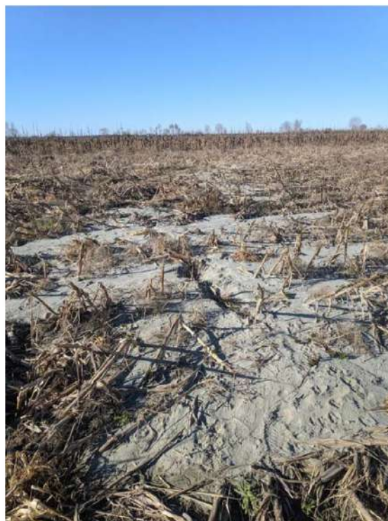
FIGURE 8. EXAMPLE OF LIQUEFIED SAND IN THE FIELDS SW OF RRUSHKULL.
