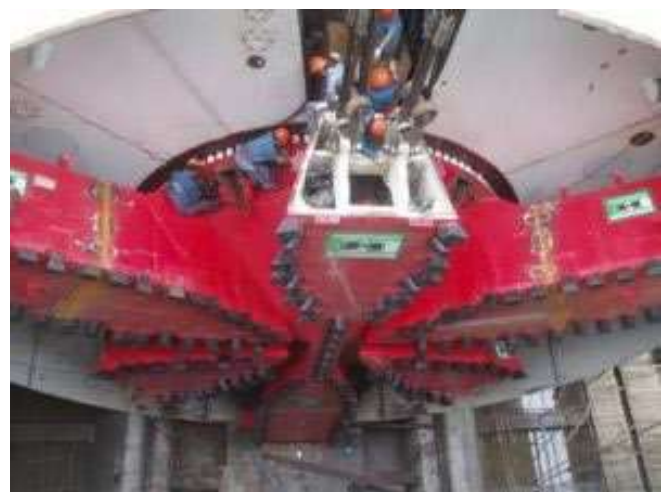
Chong Ming South TBM: Person-Entry Through Cutter Head Spokes for Cutting Tool Changes
