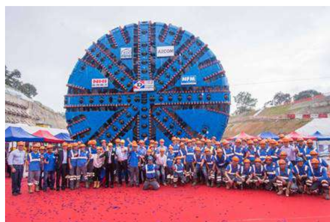
Liang Tang Tunnel: 58ft Dia EPB TBM
