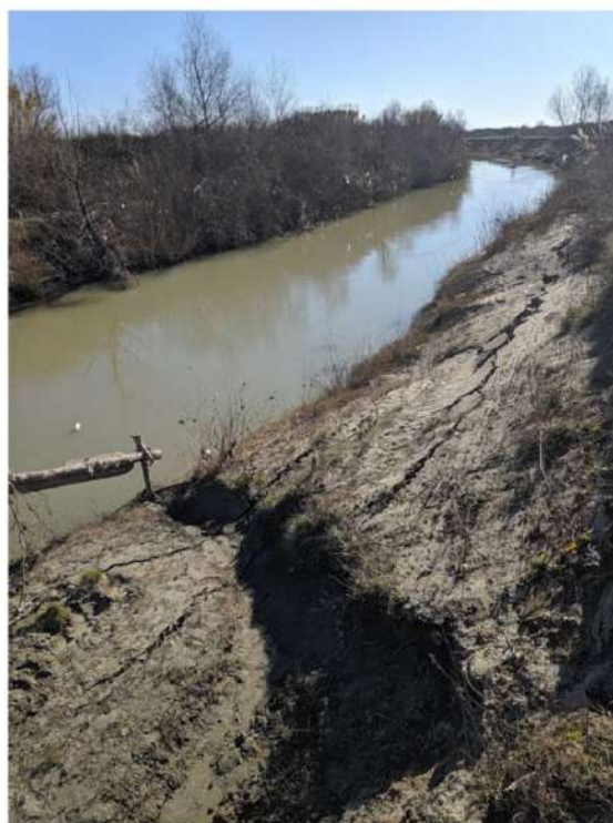
FIGURE 10. LATERAL SPREADING ALONG THE RIVERBANKS IN RRUSHKULL AREA.
