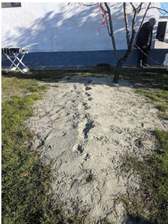
FIGURE 7. SURFACE RUPTURE AND EJECTED SAND.
