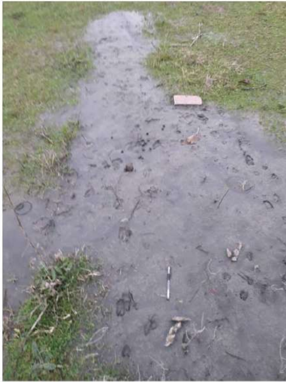
FIGURE 17. LIQUEFIED SAND IN GURËZ AREA.
