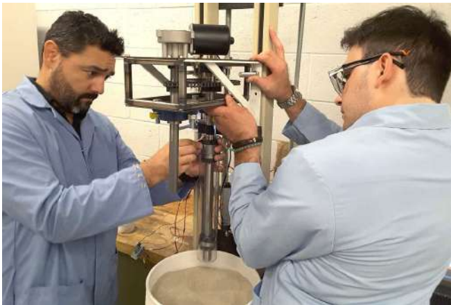
New Mexico State University associate professor Douglas Cortes, left, and Russell Buehling, undergraduate research assistant and electrical engineering senior, prepare a bio-inspired self-excavating probe for testing in dry sand.
