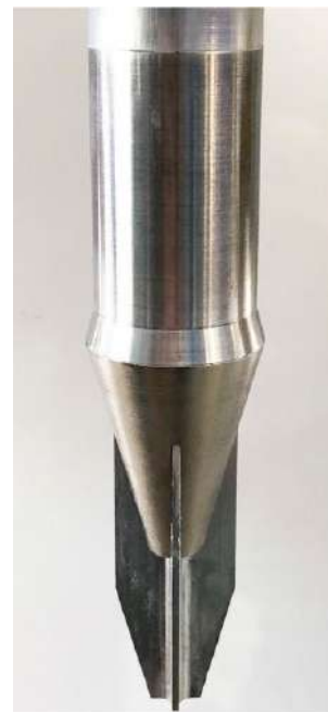
Figure 5. Stinger cone with deployable vanes for near-surface and deep penetration.
