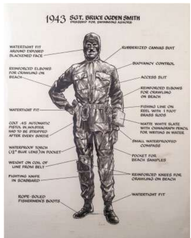
Figure 4. COPP operational attire (drawing). One-piece overalls-styled protective suit with fitted hood and external pockets, worn by COPP-1 team members.
