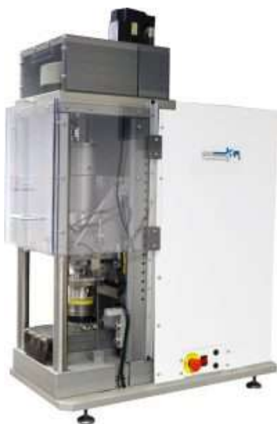
Figure 3: The GDS Electromechanical Dynamic Cyclic Simple Shear (EMDCSS) device
