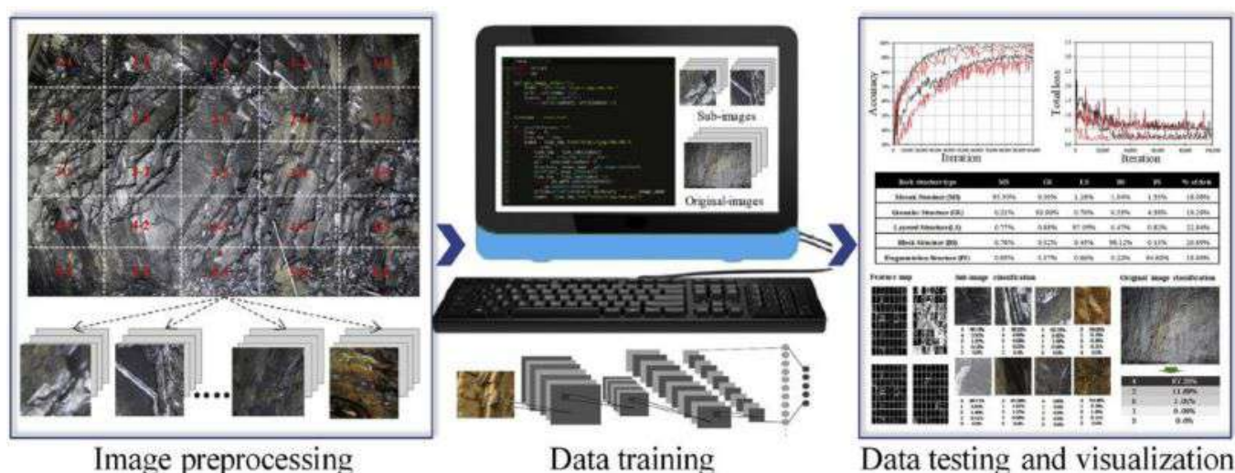
Fig. 10. Schematic diagram of rock tunnel face structure classification processes based on the proposed method.
