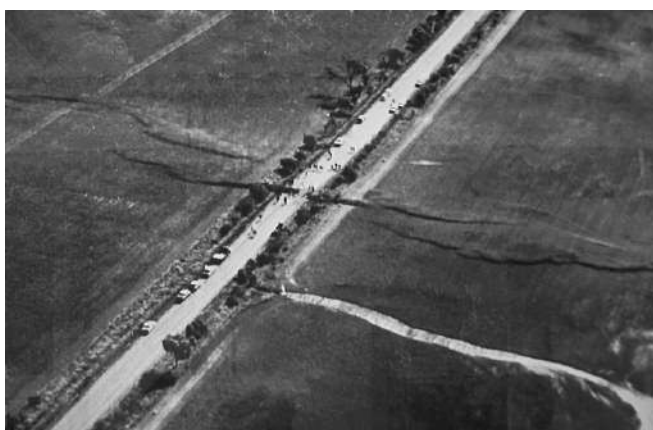
Aerial view of a more than 30km long surface rupture observed in Meckering Western Australia in 1968 as a result of 6.6 magnitude earthquake.
