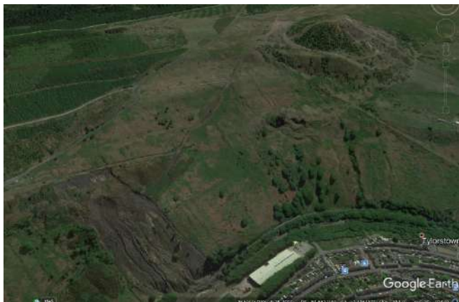
Google Earth image of the coal waste tips at Tylorstown in South Wales. Note the large conical tip at the top of the hill and the failed tip in the lower left corner.
