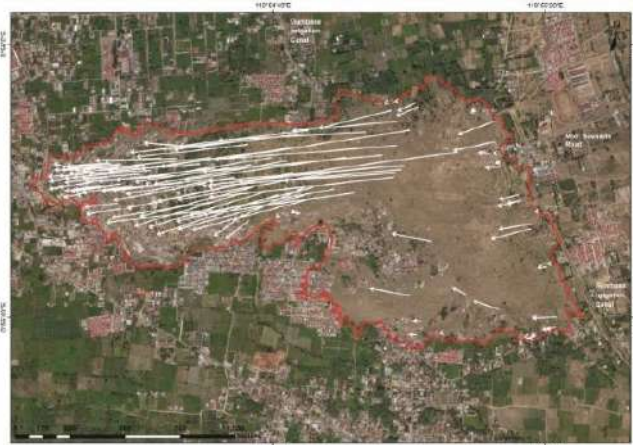
Movement vectors for the landslide at Petobo in Indonesia. Figure from Kusumawardani et al. (2021) .
