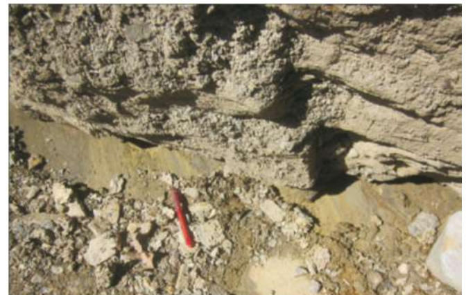
Slide surface observed during the site investigation
