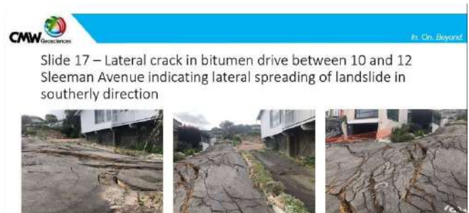
Ground deformation in the Mira Mar landslide in Albany, Australia. Image from a geotechnical report by CMW Geosciences .
