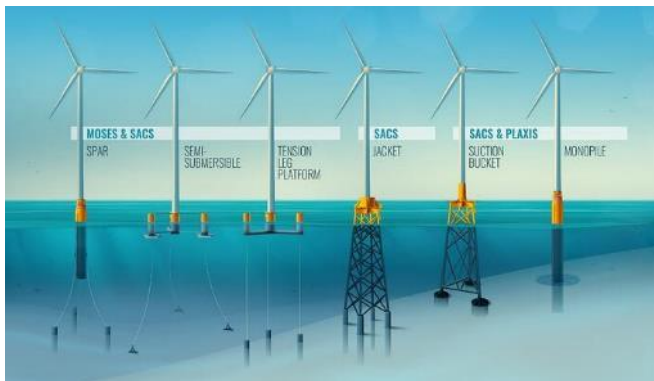
Figure 5: Types of wind turbine foundations, and Bentley software to address each type of foundation.
