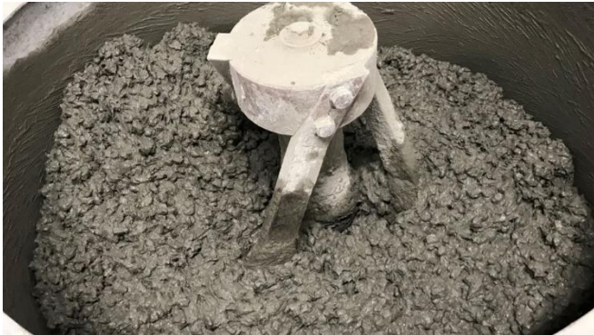
Concrete mixing using recycled tyre rubber particles for the complete replacement of traditional coarse aggregates - Mohammad Islam, RMIT
