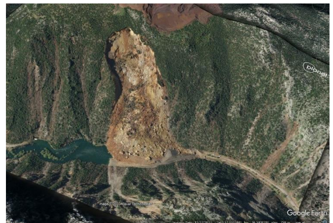
Satellite image of the valley-blocking landslide near Islahiye, Turkey, draped onto the Google Earth DEM. Image copyright Planet , used with permission. Image dated 5 April 2023.
