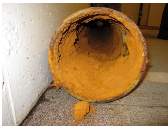
Figure 3 – Iron ochre buildup in sub-grade drainage system pipe
