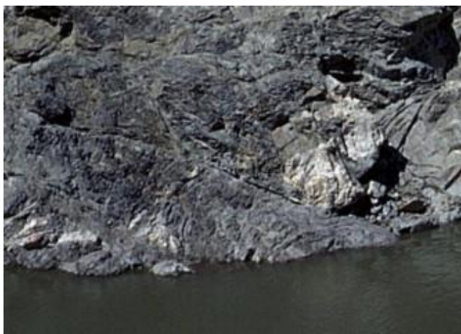
Fig. 6. Close view of a cross section of the main fault on right bank. The finely crushed borders of the fault zone are well visible, thickness about metric (photo Duffaut, 1960).
