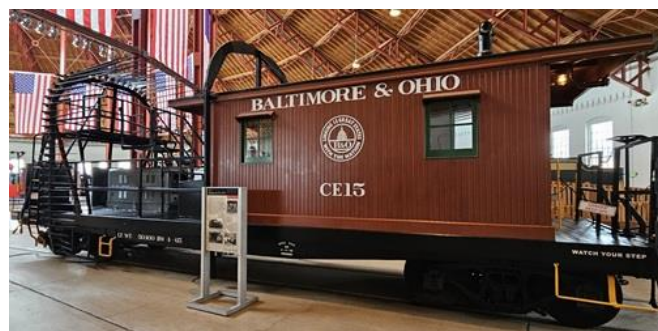
Image 8: B&O clearance car used to inspect vertical and horizontal clearances of the railroad's tunnels, B&O Railroad Museum. Source: Author.
