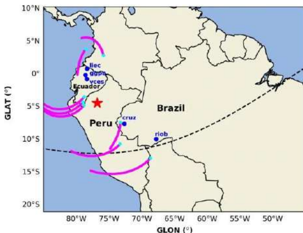
Locations of GNSS receivers are marked by blue dots. Magenta lines represent the IPP trajectories for GPS satellites 2, 5, 15, and 24, while cyan diamonds indicate the IPP at the time of the earthquake (10:52:14 UT). The red star marks the epicenter of the earthquake. The dashed curve, extending from west to east, represents the geomagnetic equator. Credit: Pre-seismic ionospheric disturbances (PIDs) associated With 2021 Mw 7.5 Northern Peru earthquake: GNSS and ground uplift observations, Oluwasegun M. Adebayo et al.
