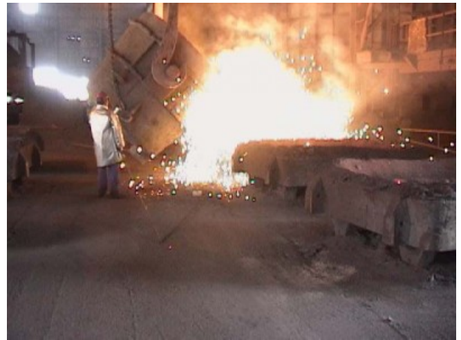
Geopolymer mould used in steelmaking, showing temperature resistance at over 1400C – Air Force Office of Scientific Research.
