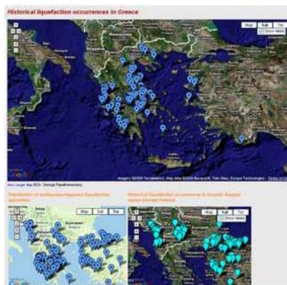
Figure 7. Home page of DALO v1.0 showing the three compiled maps of liquefied sites in Greece and surrounding countries and the earthquake-induced liquefaction epicenters.
