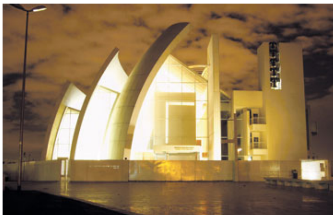
DAVIDE LUSSETTI : Rome's Dives in Misericordia Church was one of the first buildings to use a special form of self-cleaning photocatalytic concrete.
