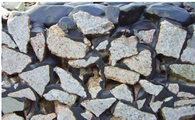
Polymer-coated ballast has been used on rail track, but it has yet to be tested on a bridge.
