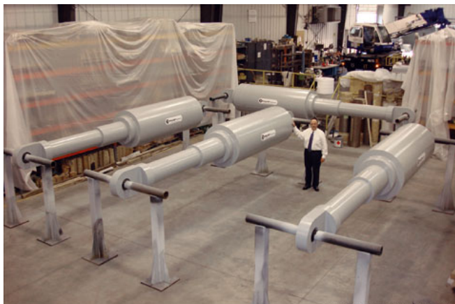
Douglas Taylor, CEO of Taylor Devices, stands next to earthquake shock absorbers used on the Sutong Bridge in China, a 4.7-mile long cable suspension bridge.
