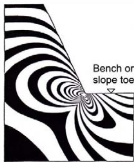
Figure 61. Stress concentration at the bench or toe zone of a slope. Results from photoelastic model tests (Hoek, 1969).
