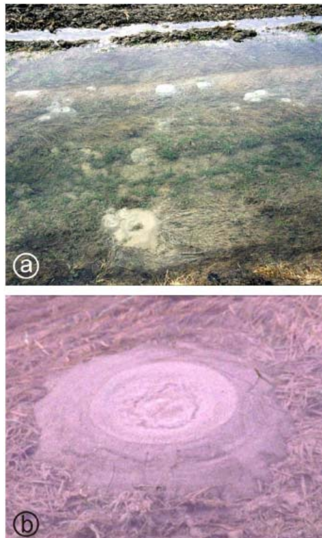
Figure 3. “Boiling” behind dykes indicates inner erosion and beginning of hydraulic failure. a) randomly distributed multiple boiling; b) detail of an erosion spot.
