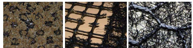
Figure 84. Geosynthetics (a, b) and wire mesh (c = right) to prevent damage to flood protective dams caused by beavers. Field tests in cooperation with zoologists.
