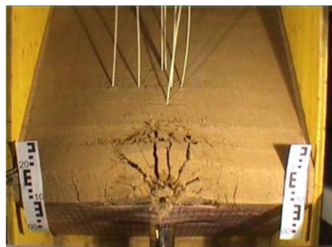
Figure 30 a, b. Cracks in a non-reinforced/reinforced model caused by the impact of the rockfall pendulum.
