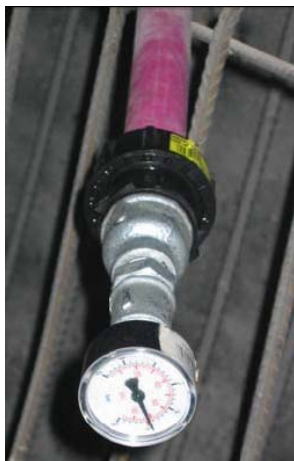
Figure 77. Tightness control after finishing all welding work at the pipe system.
