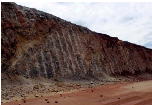
Pre-splitting – once used only on final batters now being used for rockfall control on production batters adjacent to haulage routes
