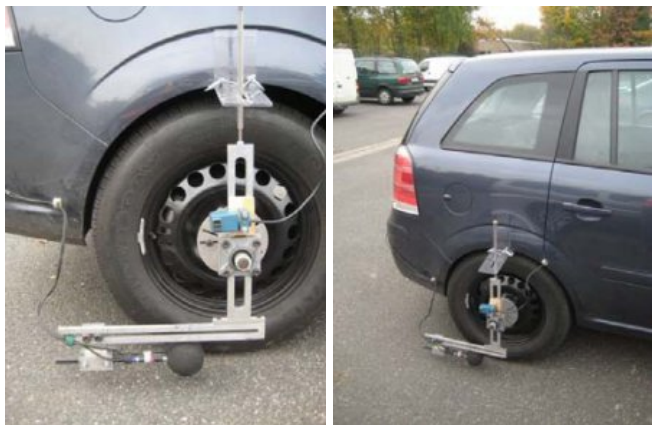
Figure 6 – OBSI bracket and test vehicle (Opel Zafira)
