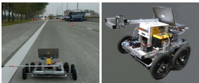
Figure 7 – RoboTex three-dimensional pavement texture measurement system
