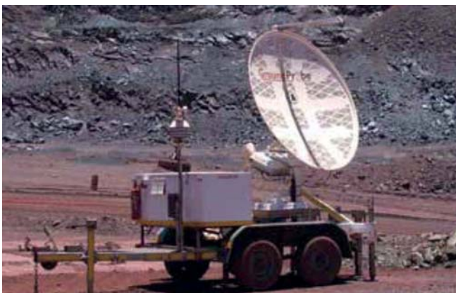
GroundProbe SSR (Slope Stability Radar)
