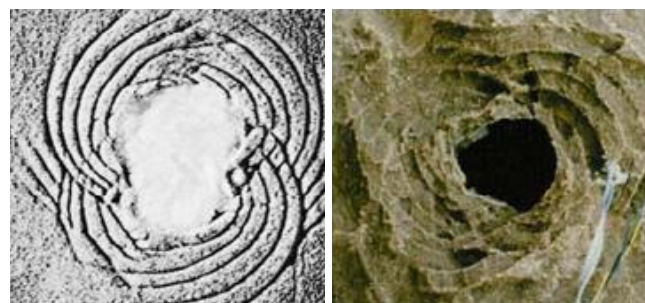
Figure 6. Log-spiral shearing with a 45° inclined hole drilled in the direction of \sigma_H into a stressed block of model sandstone, with principal stress ratios \sigma_v = 1 , \sigma_H = 0.8 , \sigma_h = 0.4 . Addis et al. , 1990.
