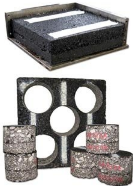
Double-layered slabs prepared with Roller Compactor and ASTRA device (UNI/TS 11214)
