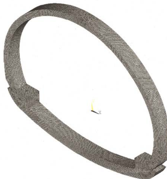
Figure 26. 3-D finite element model of the tunnel final lining
