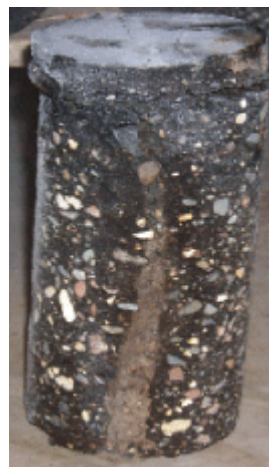
Lab examination of core displays thermal crack, a problem of HMA mixes in cold-weather regions
