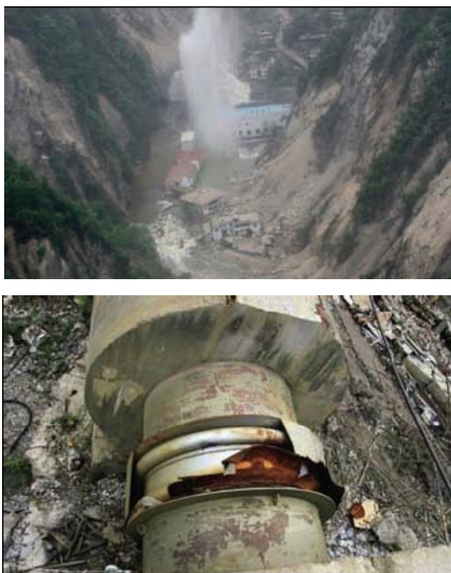
Figure 7. Failure of penstock near Shapai powerhouse: Water jet from failed expansion joint and flooding of powerhouse area (up) and detail of damaged expansion joint (down) (Wenchuan earthquake, China).
