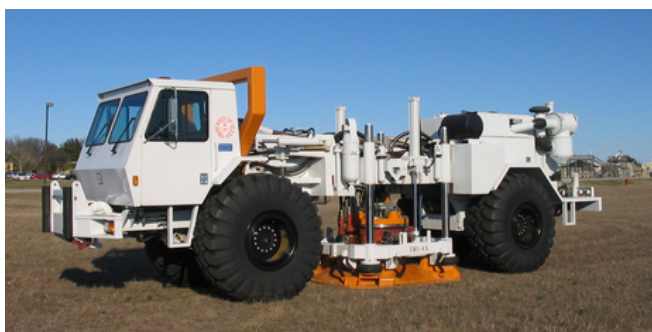
The T-Rex truck thumps the ground to help simulate an earthquake. Photo / Supplied
