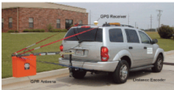
GPS-enabled survey vehicle incorporating ground penetrating radar.
