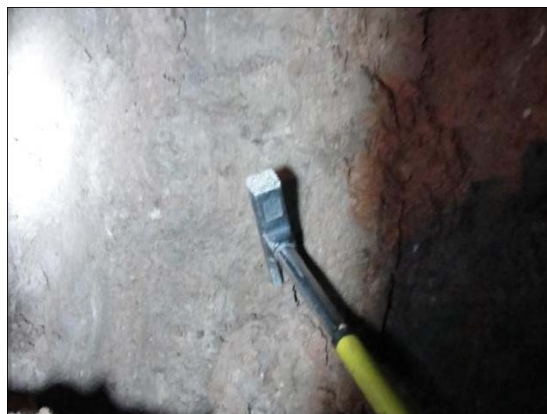
The impermeable clay cap over the salt in the Ionakhsh fault
