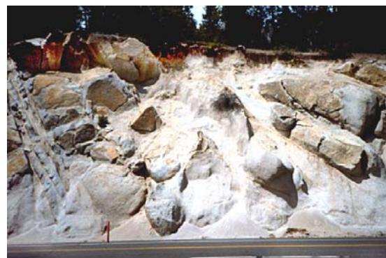
Figure 1: Decomposed granite: a weathered rock located in the Sierra Nevada mountains of California. Hard blocks (corestones) surrounded by "gruss", granite completely decomposed to dense sandy soil. (Photo: E. Medley).
