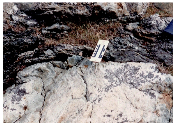
Figure 5: Weakest element in a bimrock is generally the block/matrix contact. Gwna Melange, Anglesey, Wales. (Photo: E. Medley).
