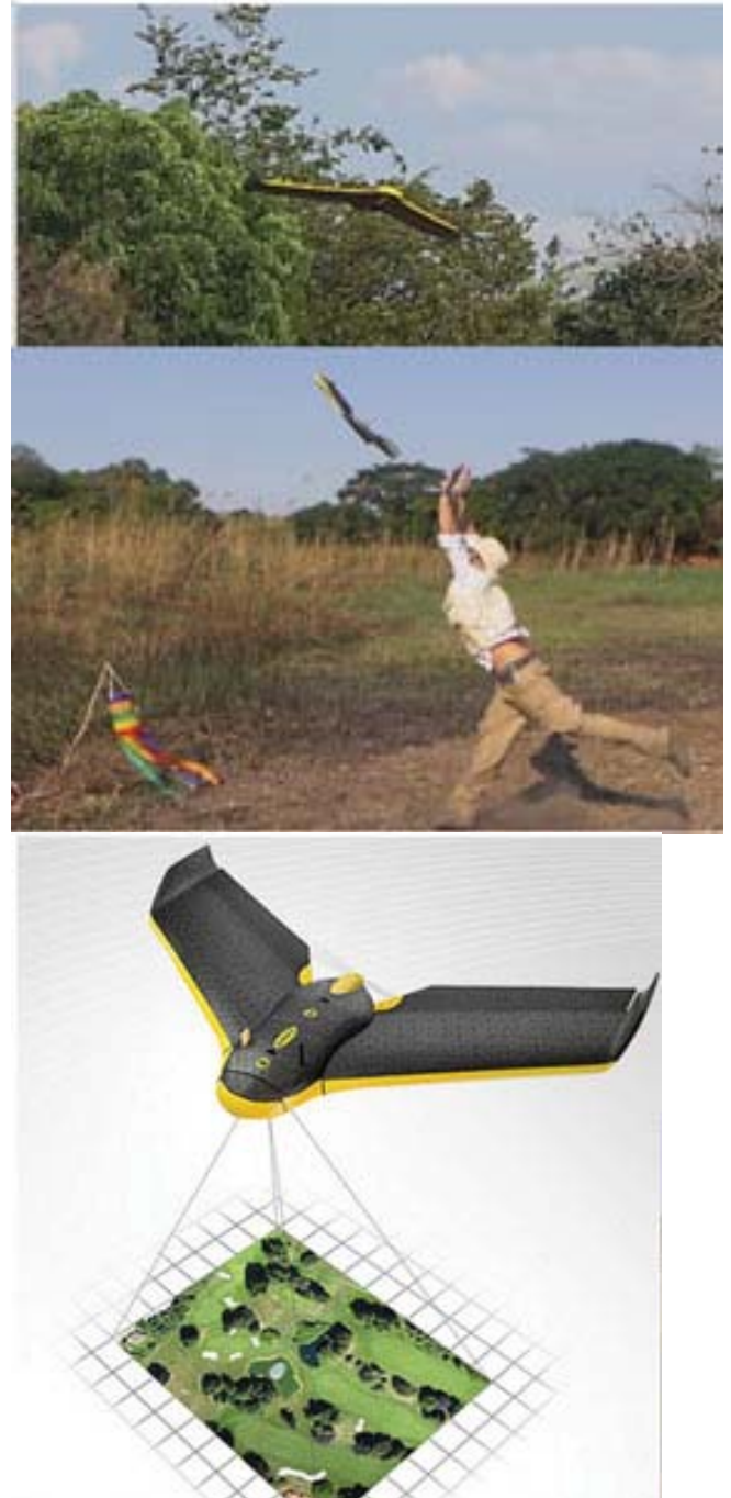
Drones were deployed equipped with a camera and various sensors to prepare detailed geo-referenced ortho photos, digital terrain models, contour lines and additional data.
