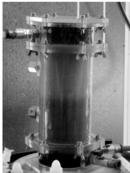
**Figure 2.** View of dyed colloidal silica at (approximately) midheight of sand sample during test No.4.
