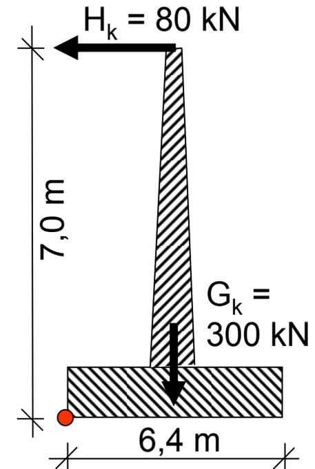
With this enlarged footing verification of reinforced concrete structure of the footing can be done with a (fictive) ground pressure distribution within the area of the footing
