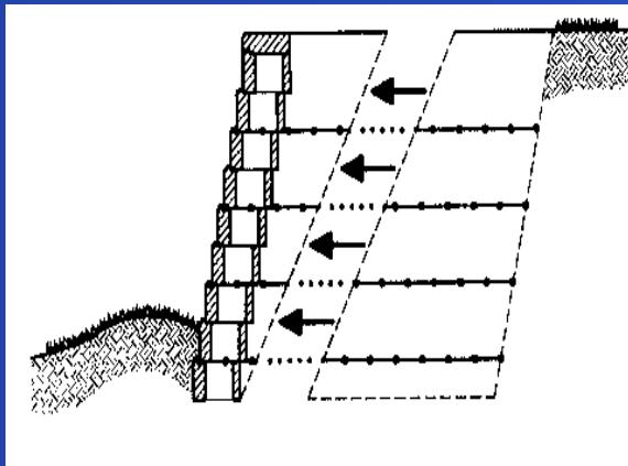
**Failure of reinforcing
