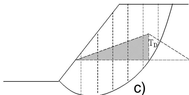
**Assumptions for reinforcement implementation into stability calculation**
